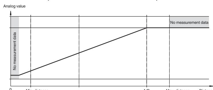
**Rising slope (A < B)**
